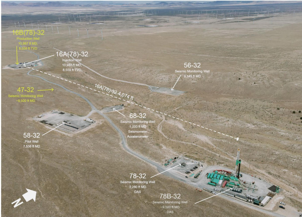
Figure 2: Aerial view of surface locations of Utah FORGE wells. The primary purpose of well 78B-32 is to provide a site where R&D tools and technologies for EGS development can be tested. At other times, the well will be used for seismic monitoring.
